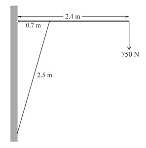
A uniform beam has length 2.4 m and weight 68 N. The beam is hinged at a fixed point of a vertical wall, and held in a horizontal position by a light rod of length 2.5 m. One end of the rod is attached to the beam at a point 0.7 m from the wall, and the other end of the rod is attached to the wall at a point vertically below the hinge. The beam carries a load of 750 N at its end (see diagram).
